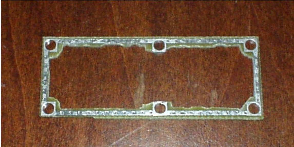
Figure 10: Spacer section, after being cut away from the raw PCB and milled out.
